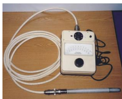
The Siemens-Reiniger-Weke "Universal-Dosimeter" dosimeter with the normal ionisation chamber, designed in 1938, introduced to radiotherapy departments after the Second World war.
