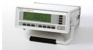
The PTW-Freiburg UNIDOS E Universal Dosimeter , produced in 1992.
