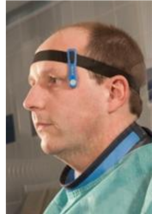
Eye lens dosimeter worn at representative position
